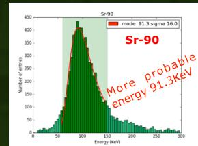
**EXERCISE 5:** gets the energy deposition of a minimum ionization particle (*mip*) in 300μm of silicon.
