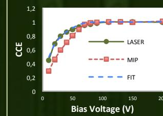
**EXERCISE 9:** the CEE of a *mip* and an absorbed 980nm laser beam are compared. The laser penetration is calculated.
