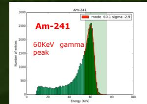
**EXERCISE 10:** a self-trigger is used to determinate the energy of particles fully absorbed in 300μm of silicon.
