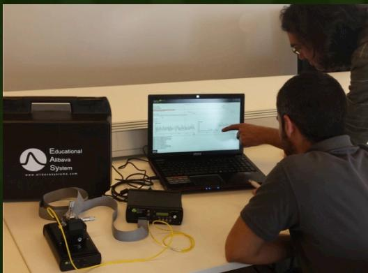
The **EASY** system illustrates the operation of a silicon strip detector with LHC readout electronics in **10 EXERCISES**.
